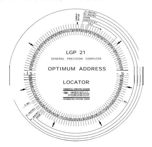
FIGURE 8.3 Optimum Address Locator
