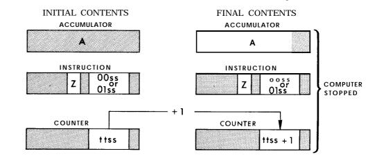
When n = 0200 or 0300, no operation occurs; i.e., the computer does not halt, the contents of the Accumulator remains unchanged, and nothing in memory is altered.
