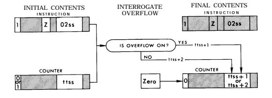
If Sense Overflow is combined with Stop (-ZOOOO), the skip or no skip is deferred until after the stop. If no Branch Switches are to be tested and no stop is desired, the track address can be 02 or 03.
