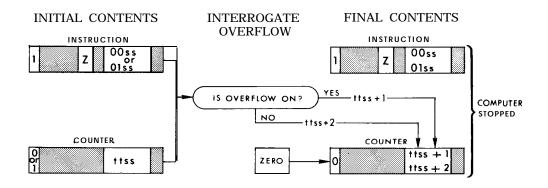
Overflow and/or any combination of Branch Switches can be interrogated with one Sense and Transfer instruction.
