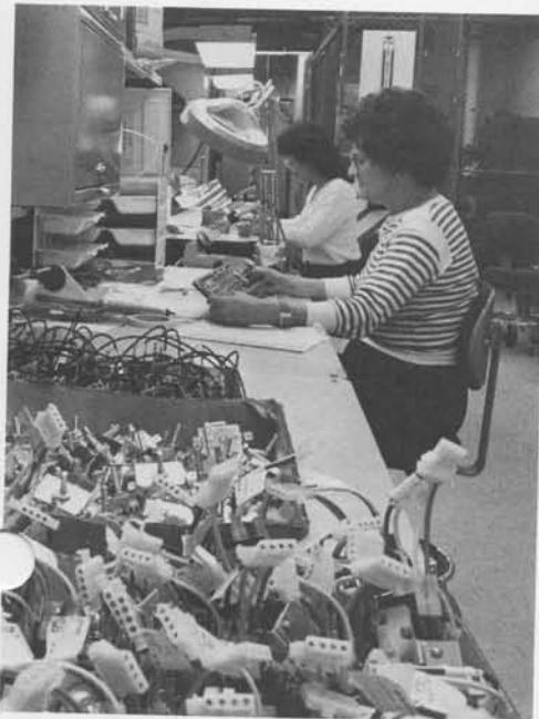
A large part of computer manufacturing is not robotized, but people assemble, wire and test the components that make up a machine. This photo is from a Data General prototype assembly plant in Westborough, Massachusetts.
