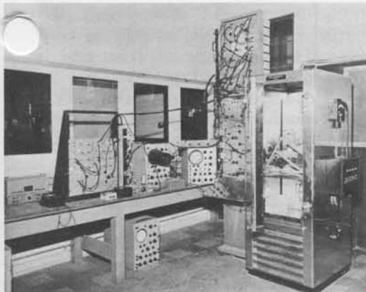
**Electrical Testing.** Core drivers helped in electrical core testing. The cores, which were temperature sensitive, were tested at a uniform 25 C. The temperature was controlled by core handlers in temperature-regulated boxes or air-conditioned rooms.
