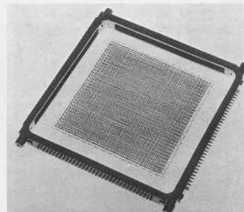
**Finished Product.** The final operation in the construction of a plane was the insertion of the inhibit winding and sensing wire which linked all the cores in the plane.
