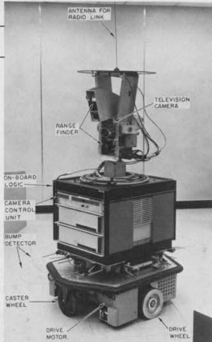
The Computer Museum has a new found friend named Shakey. Developed in 1969 by the Stanford Research Institute, Shakey was the first fully mobile robot with artificial intelligence. He was not named until fully operational, and then named himself by his "shakey" actions. Shakey is seven feet tall with his antenna, has a TV camera, and touch and distance sensors. Shakey will be on exhibit in our new home at Museum Wharf.
