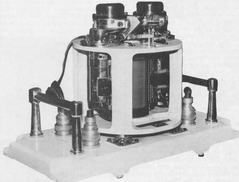
Drum from the English Electric Deuce. Built in 1957, the Deuce drum stored  $8K \times 32$ -bit words on 256 tracks of 32 words each. It measured four inches by six inches; most first-
