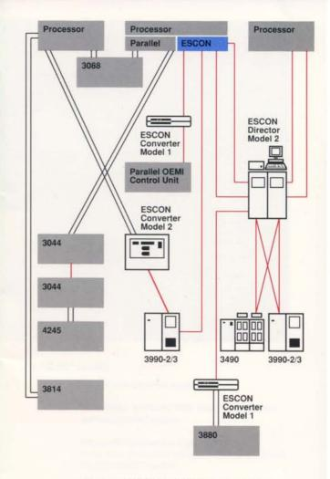
ESCON Channels and parallel channels attached to the same control unit have to be on different images. If you use two ESCDs in tandem, only one will provide dynamic connectivity; the other will be static.
