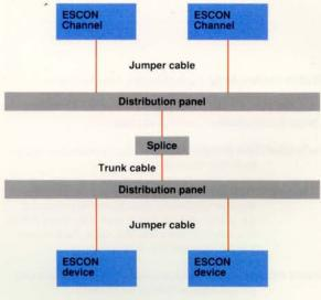
An **ESCON device** can be an ESCON Channel, an ESCON control unit, an ESCON Director or an ESCON Converter
