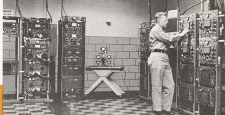
AN AIR FORCE OPERATOR tunes radio equipment used for the voice control of manned interceptors.
