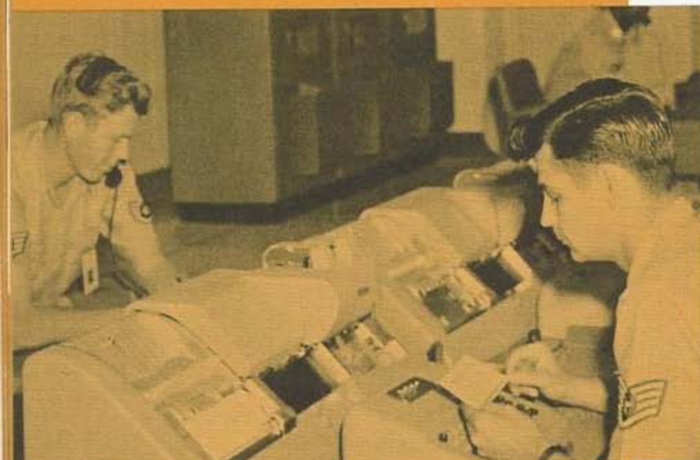
AIR FORCE OPERATORS in the manual inputs room insert flight plans, weather data and other non-automatic data into the computer at the Direction Center.
