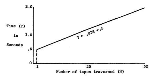
Figure 2. Approximate Read-Write head movement time
