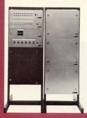
Indicator Panel – displays all important data registers and control latches.
