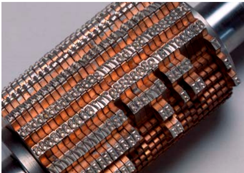
15. Stereotype Punches for Difference Engine No. 2, 2002. (Science Museum, London)
