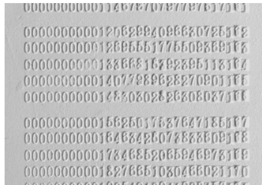
16. Stereotype Mould in Plaster of Paris, for Difference Engine No. 2, 2002. (Science Museum, London)
