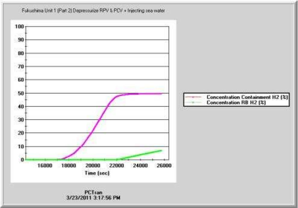
Hydrogen in the Reactor Building reached detonation point (5%) and exploded.
