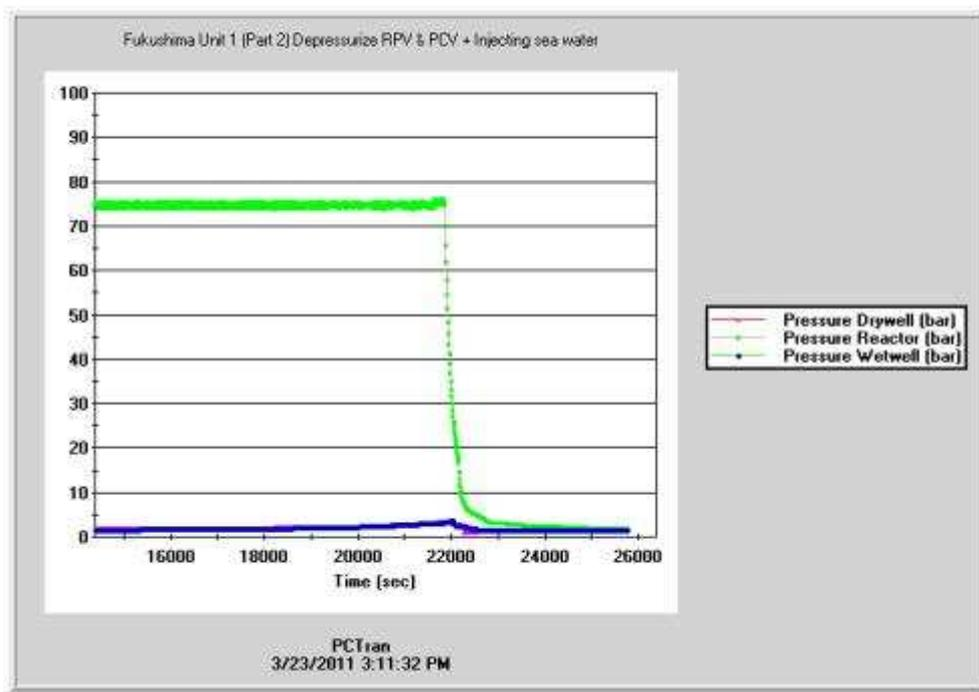
Operator depressurize the RPV and PCV to vent hydrogen
