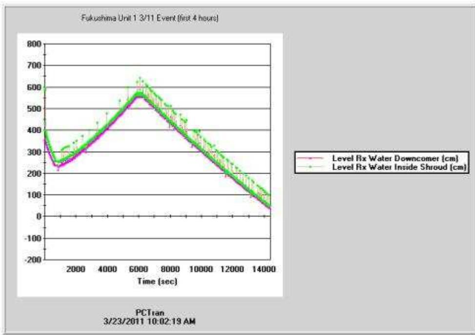
Reactor water level above top of active fuel – RCIC started at 600 sec to makeup SRV loss; terminated around 6600 seconds so the level dropped.
