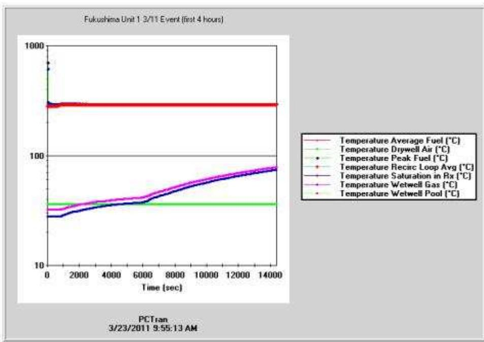
Fuel and reactor coolant temperatures stable after reactor trip; suppression pool and air temperatures heated up by SRV steam discharge; drywell air temperature increased slightly by flipping of the vacuum breaker between drywell and wetwell.
