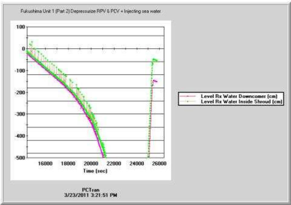
Water level (above top of active fuel) in the RPV; sea water and borated water was used to recover the core.
