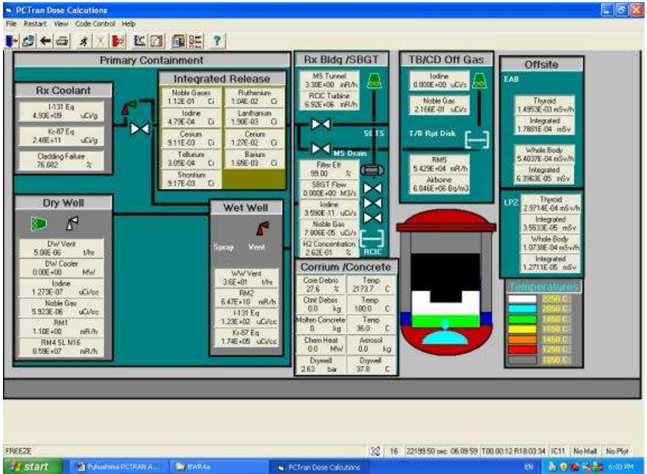
Containment and radiological release mimic displays core collapsed condition; note operators have open the wetwell vent valve (color in red) to vent the containment.
