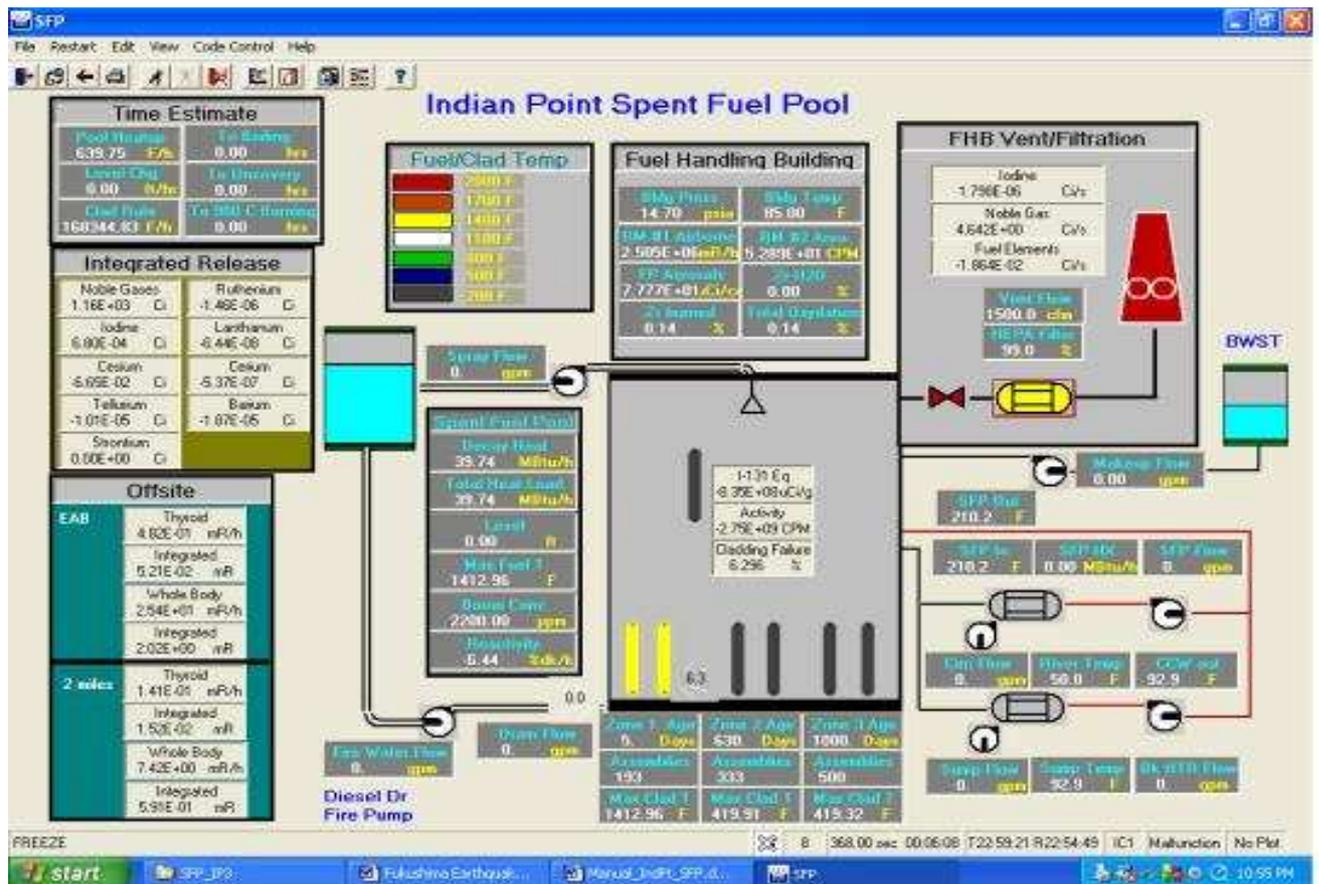
Spent Fuel Pool accident – after loss of coolant or cooling water boiled off. Note, a supplement
