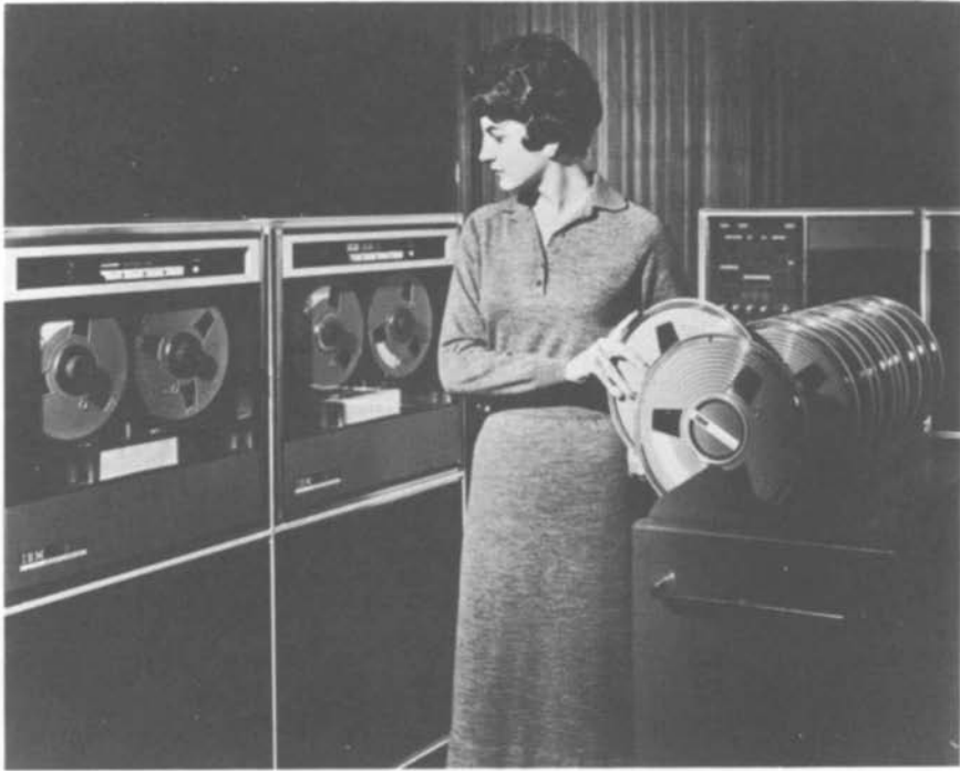
IBM 7330 Magnetic Tape Unit
