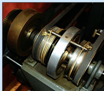
Original Nieman torque amplifier on display at the MIT Museum. This torque amplifier, based on contra-rotating capstans, amplifies the output from the integrator wheel and drives the output gears of the integrator box.
