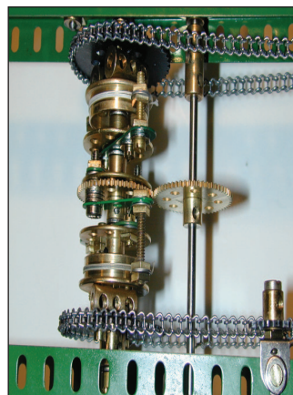
Figure 2. Torque amplifier stage. The output shaft to the left carries both rotating drums. The input shaft runs parallel on the right, carried in rotating bearings, and couples to the input arms through a pair of gears.
