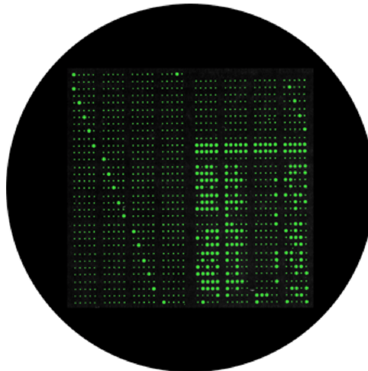
Dot pattern on the screen of a Williams memory tube of a Ferranti Mark I computer.
