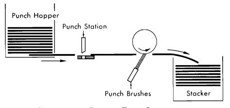
FIGURE 88. PUNCH FEED SCHEMATIC
