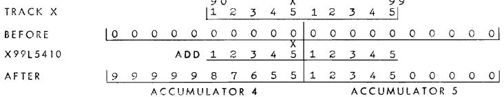
FIGURE 25. EFFECT OF SIGN CONTROL OVERPUNCH ON THE ACCUMULATORS
