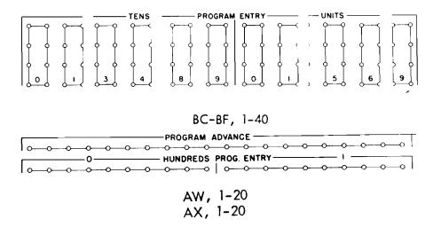
Program Entries. These hubs accept the PROGRAM EXIT impulse to set up the first step of a new sequence. Unless a new sequence is started in this manner, or by impulsing PROGRAM ADVANCE, the machine will stop.
