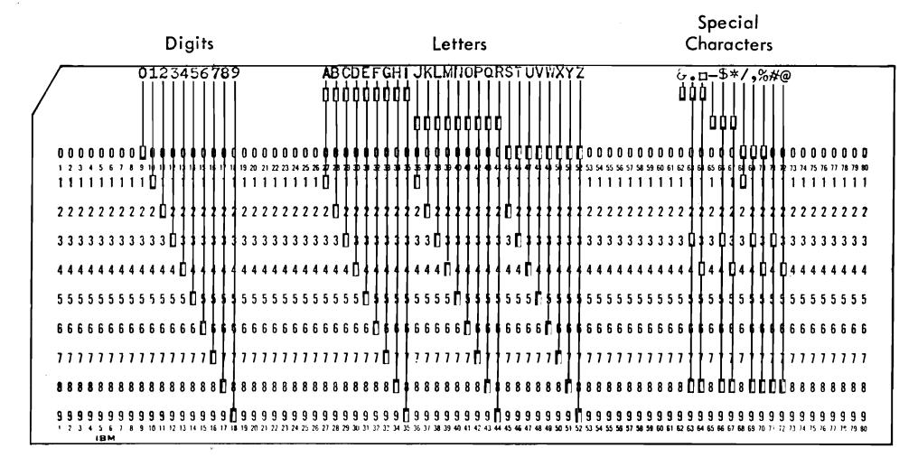
FIGURE 43. CHARACTER CODING IN IBM PUNCHED CARDS
