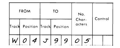
The transfer of the address to the address register requires 50 milliseconds. This instruction transmits the address of the desired sector to the address register and causes the access arm to start moving toward the disk, track, and sector specified by the address.
