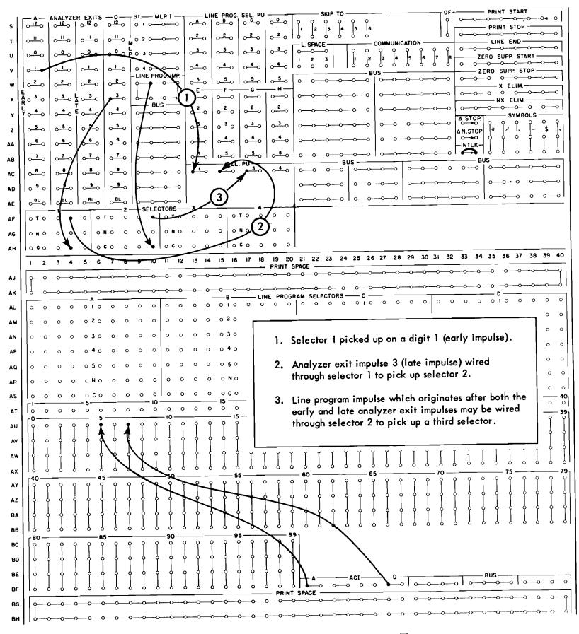
FIGURE 85. SERIES WIRING TO ILLUSTRATE TIMINGS
