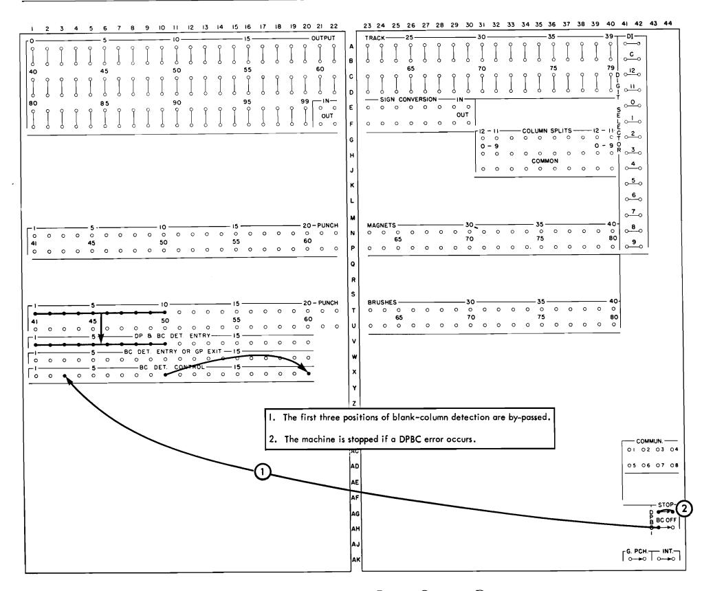
FIGURE 96. DOUBLE-PUNCH AND BLANK-COLUMN DETECTION
