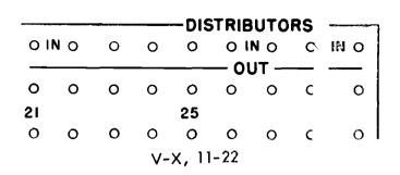
Distributors. Impulses that are used to initiate several functions are wired through distributors that serve the same function as split wires but prevent possible back circuits. An impulse wired into the IN hub of a distributor is available as the associated OUT hubs, but impulses cannot travel between OUT hubs, or from an OUT hub to the IN hub. Any impulse except that from the OUT hub of another distributor may be wired through a distributor.
