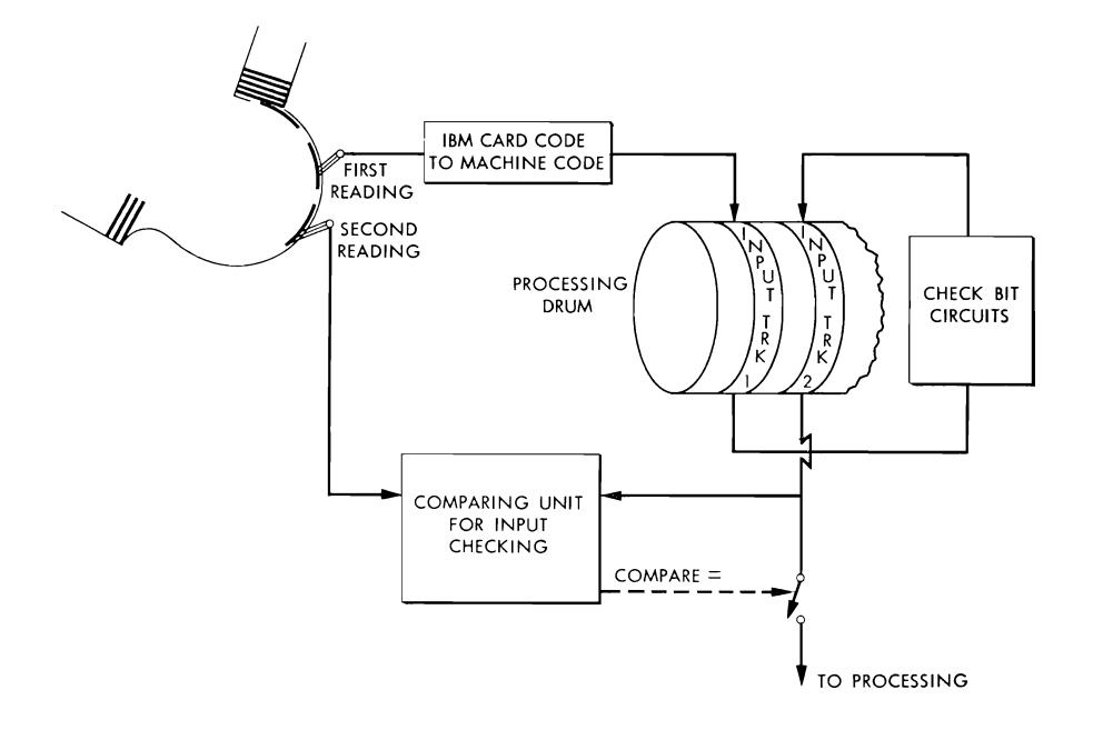
FIGURE 45. CHECKING OF INPUT CARD READING
