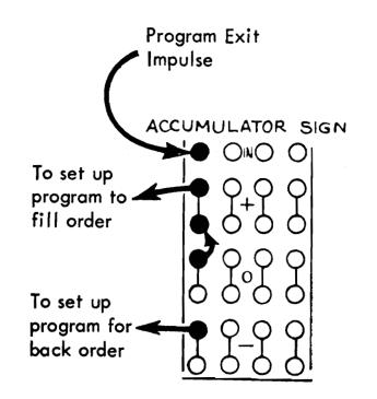
Figure 6. Method of Branching by Control. Panel Wiring
