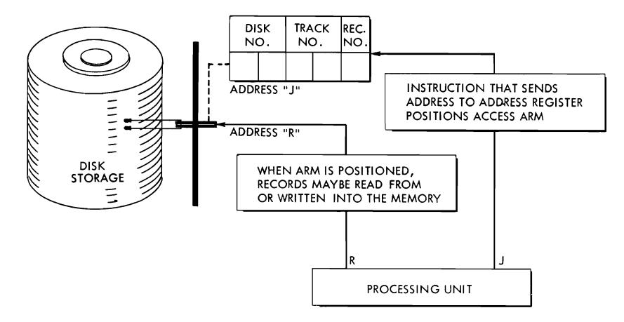
Figure 15. Method of Addressing, Reading, and Writing in the Disk Storage
