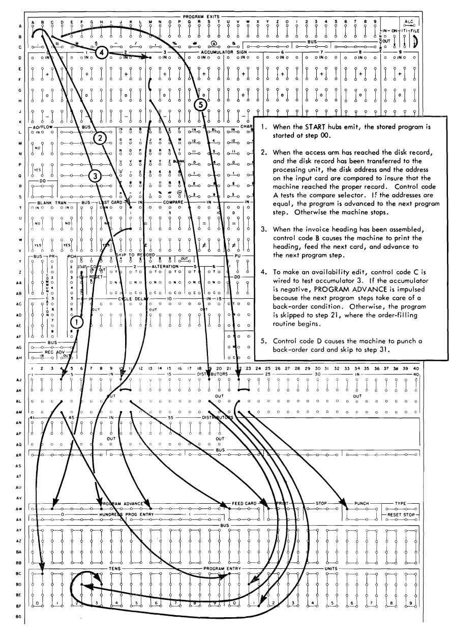
FIGURE 35. SAMPLE PROGRAM - CONTROL PANEL WIRING - PART 1
