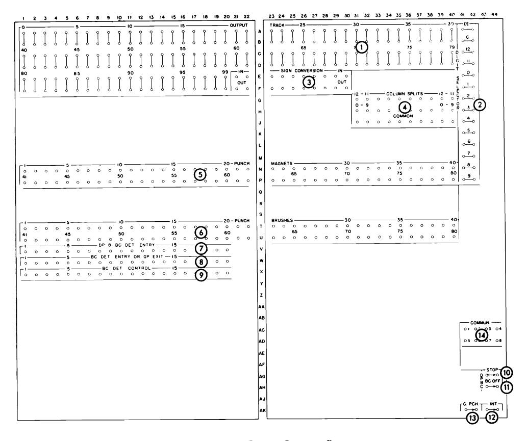
FIGURE 100. 323 PUNCH CONTROL PANEL
