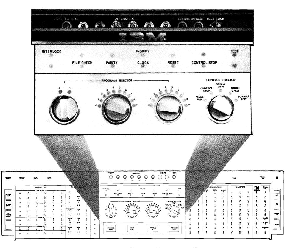
Figure 51. Control Switches, Buttons, and Lights
