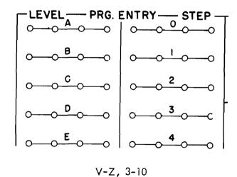
Program Entry. To establish the beginning of a sequence of program impulses, one LEVEL hub and one STEP hub are impulsed in the same manner that the PROGRAM EN-TRIES are impulsed on the process control panel. The program unit is turned on automatically by impulsing PROGRAM ENTRY, without impulsing PROGRAM ON.
