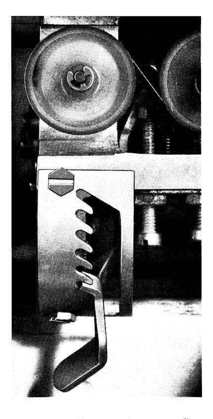
FIGURE 79. FORM THICKNESS ADJUSTMENT DEVICE
