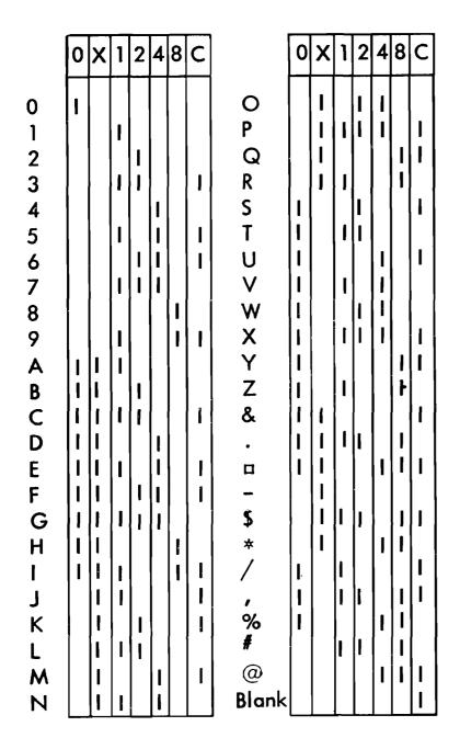
FIGURE 44. CHARACTER CODING, DISKS AND DRUM
