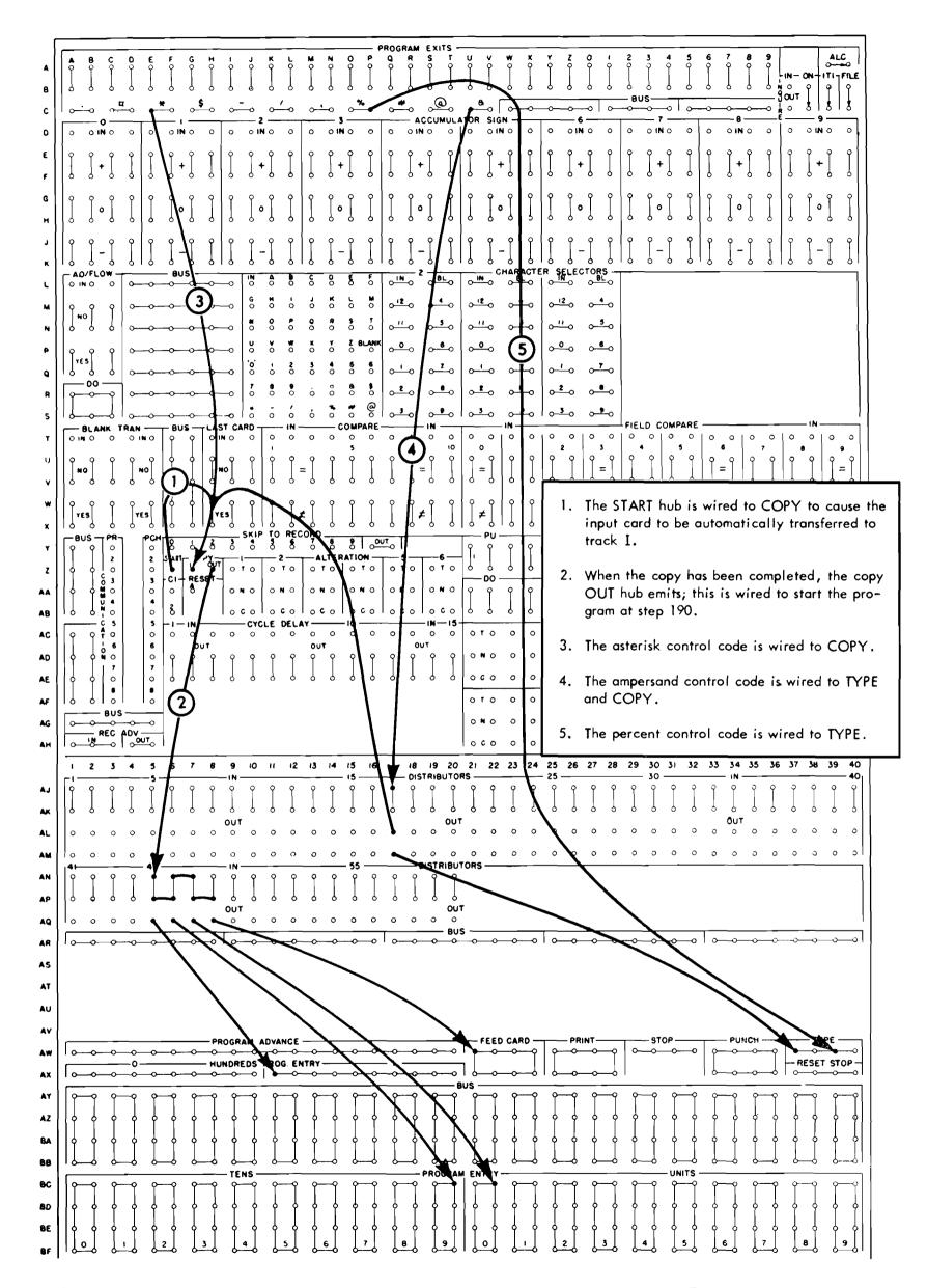
FIGURE 14. CONTROL PANEL WIRING FOR LOADING THE PROGRAM
