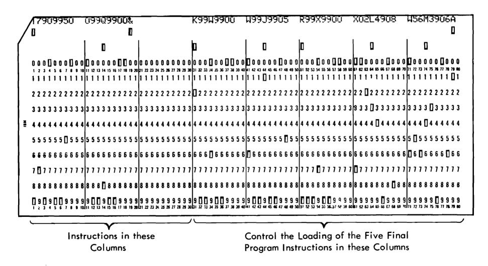
FIGURE 12. CARD USED FOR PROGRAM LOADING
