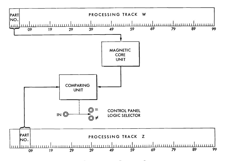
FIGURE 16. SCHEMATIC OF A COMPARING OPERATION
